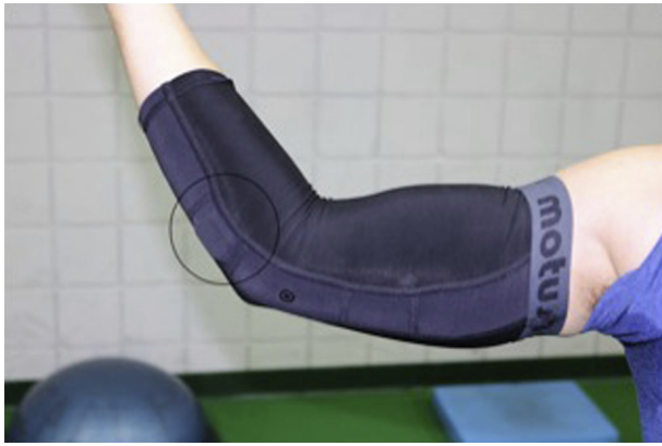
Fig 1. The compression sleeve with the elbow torque device positioned 1.5 inches distal to the medial epicondyle.
